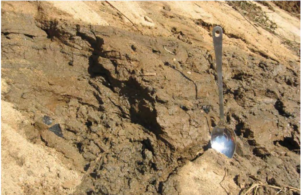
Photo 4: Bank along the north floodplain terrace, located just upstream of Woodside I Dam; stainless steel sampling-spoon is adjacent to fine grained sediment that was sampled for PCBs. Photo taken Feb. 19, 2011.
