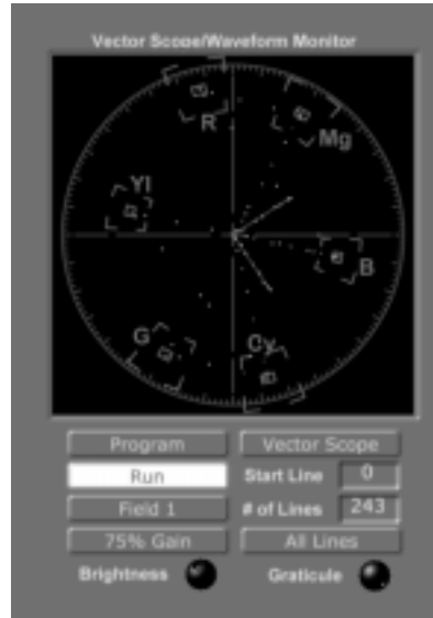
The Vector Scope, Analyzing Color Bars
