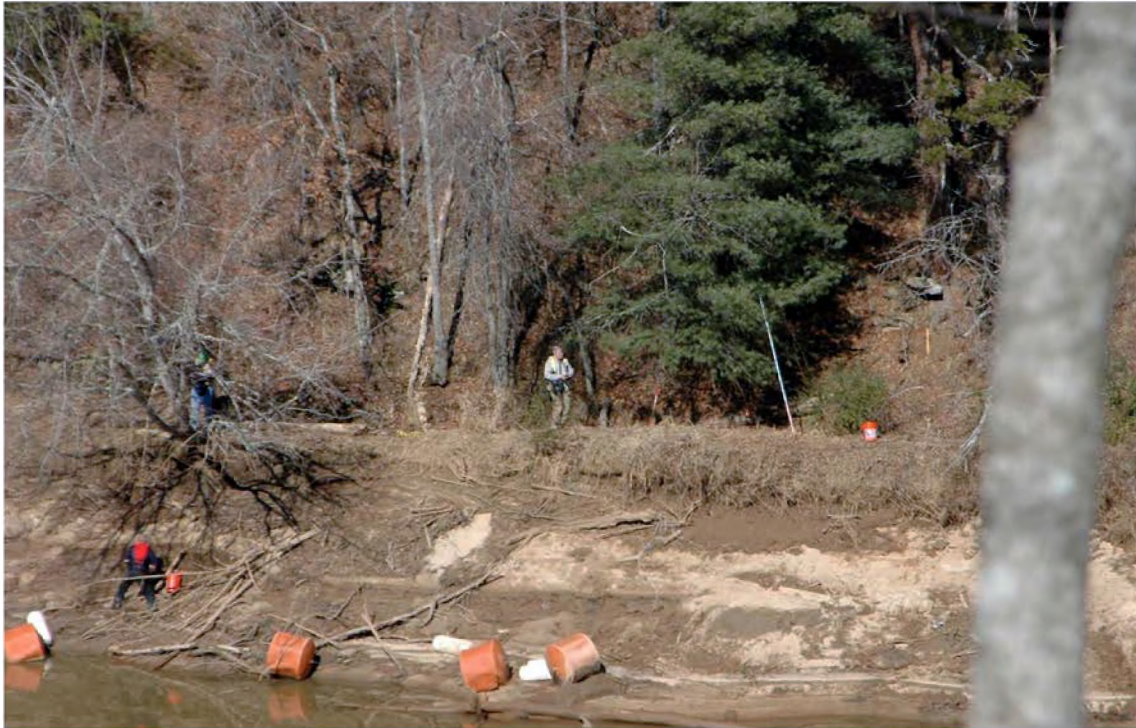
Photo 2: Sediment sampling activities on the north floodplain terrace bank, just upstream of the Woodside I Dam. Sampling focused on the dark, fine grained sediment; sampling visible in the lower left. Photo made Feb. 19, 2011
