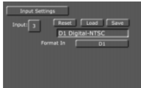
Input Settings Panel for Serial Digital Input Card
