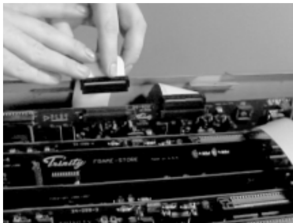
Connecting the Cables to J4 and J5 on the Time Machine Card
