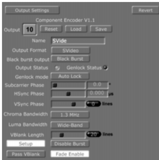
Output Settings Panel for the Multi-Format (Component) Master Encoder Card
