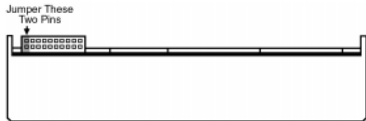
Jumper These Pins to Set SCSI ID to 1 for the Seagate Cheetah Hard Drive
