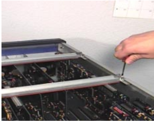
Removal of Retaining Bar
