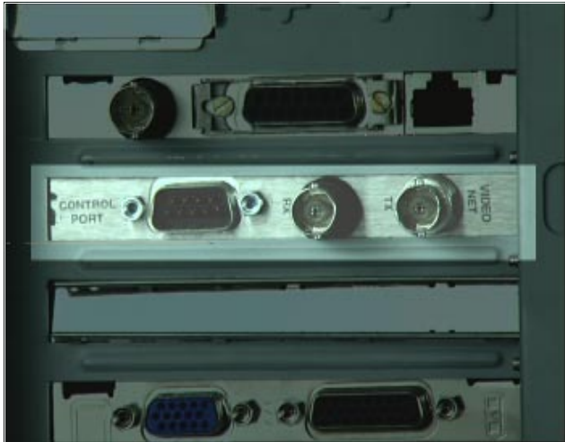
The TX And RX Connectors On The VideoNet Card
