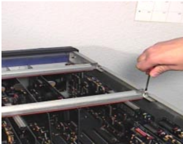
Removal of Retaining Bar
