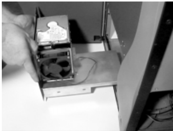
Placement of the Hard Drive Bay Unit
