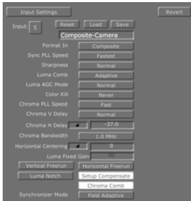
Input Settings Panel for Composite/YC Card with Frame Sync
