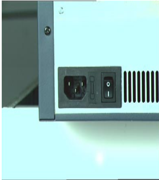
The Power Connector On The Trinity Hardware
