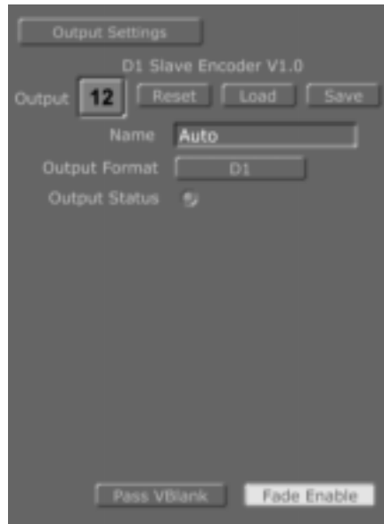
Output Settings Panel for Serial Digital Slave Output Card
