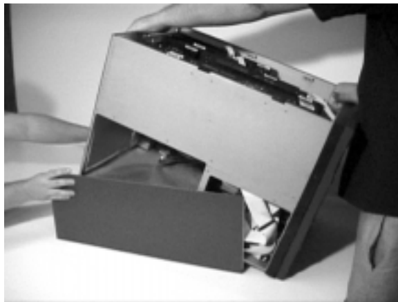
Removing the Bottom Cover of Trinity
