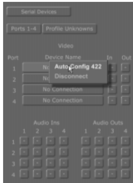
Choosing Auto Config 422 in the Serial Devices Panel
