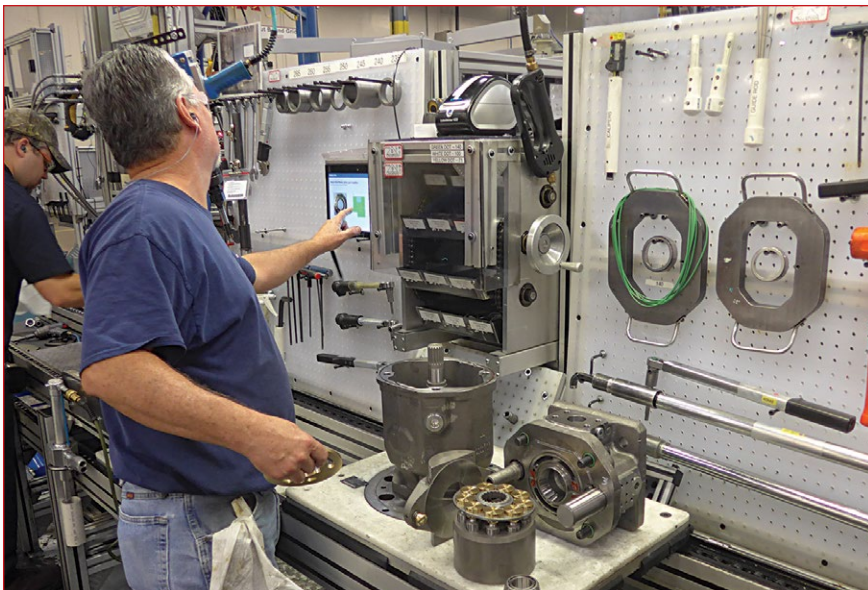
Workstations are equipped with touch screens that allow assemblers to view drawings and work instructions. Photo by Austin Weber
