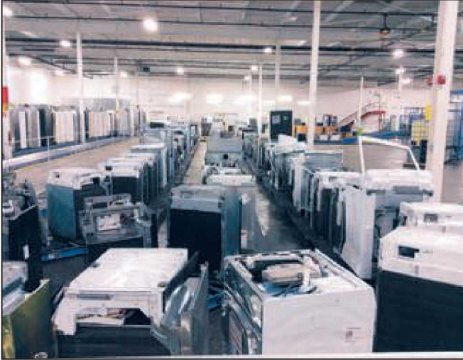
Recleim's plant disassembles household appliances into components and recycles the metals.
