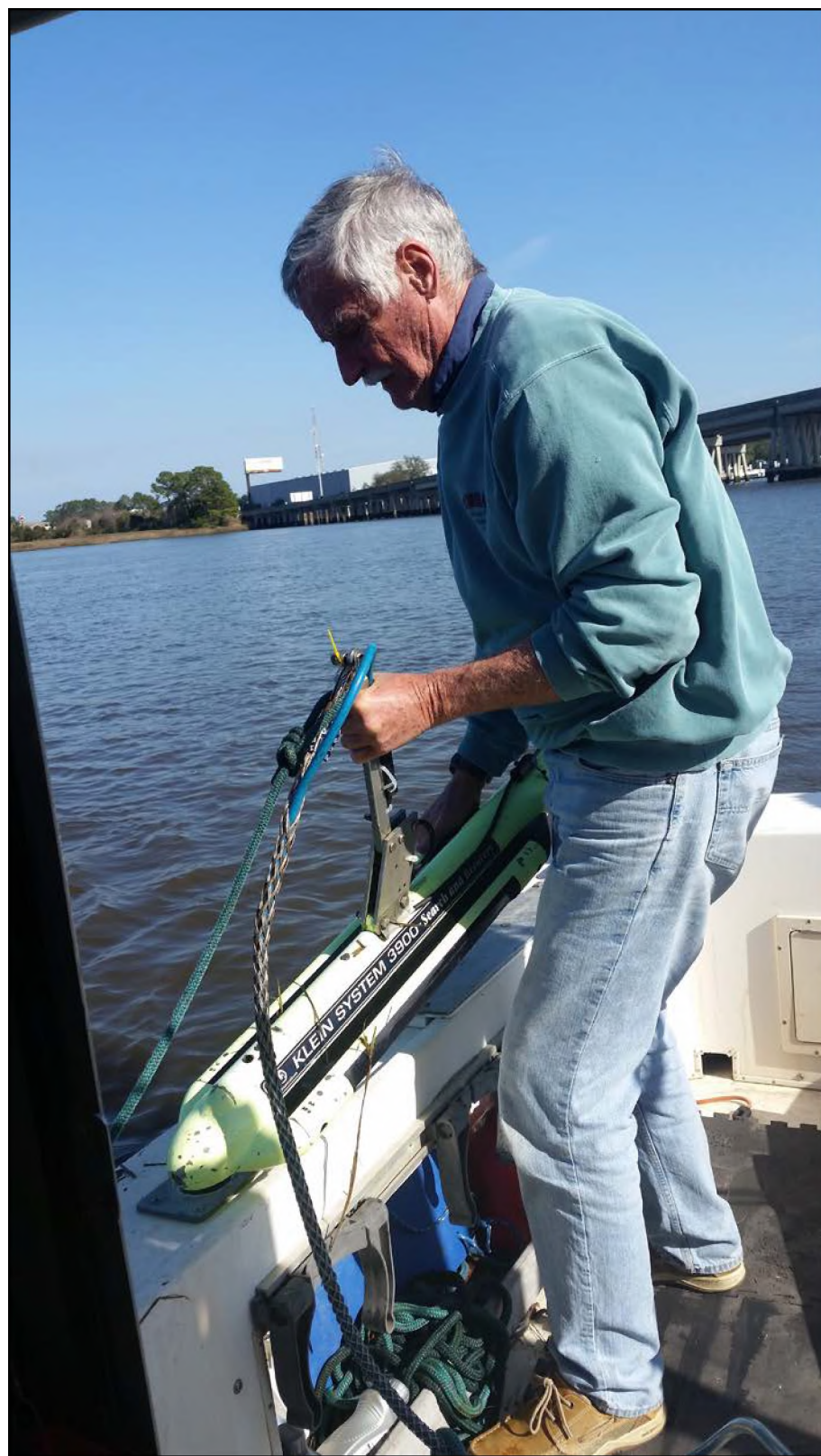
Figure 5. Rigging the Klein 3900 sidescan sonar.
