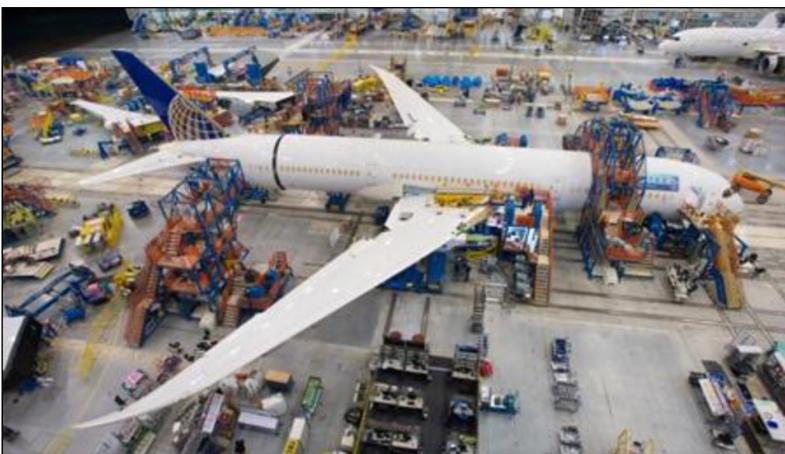
Boeing South Carolina started [final assembly on its first 787-9 Dreamliner](#). The 787-9 features a fuselage stretched by 20 feet when compared to the 787-8. The 787-9 can fly up to 40 more passengers an additional 450 nautical miles (830 kilometers) with the same exceptional environmental performance – 20 percent less fuel use and 20 percent fewer emissions than the airplanes it replaces.
