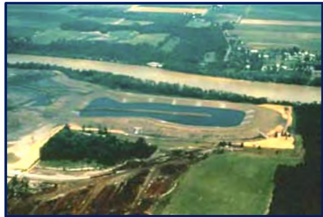
500,000 Cubic Yard Treated Hazardous Sludge Dewatering Basin/Landfill Cell
