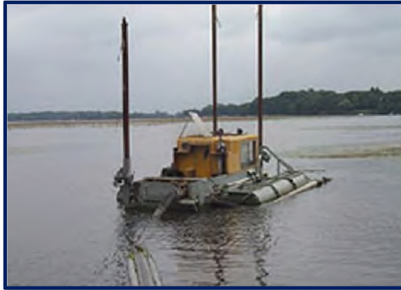
Hydraulic Dredge and Piping Similar to the Ones Used on Pheasant Branch Creek
