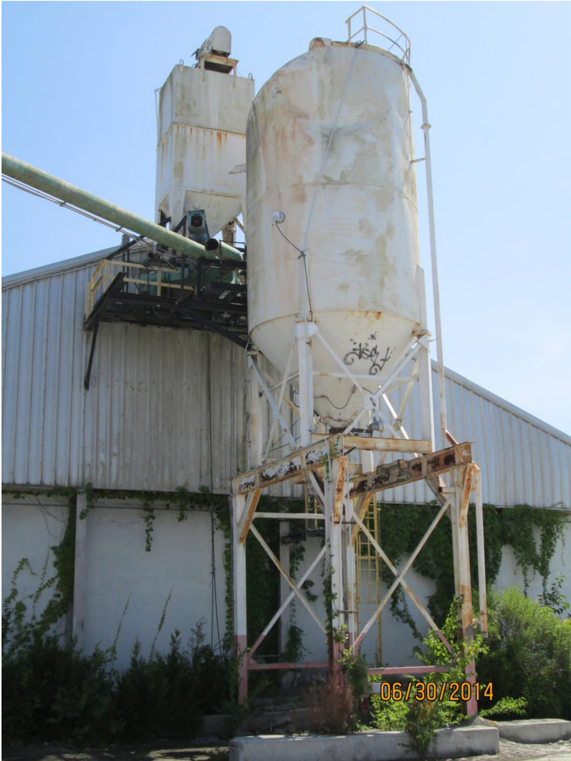
Building 2 front with cement hopper, silo, and piping, etc.
