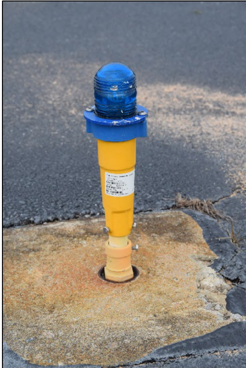
Figure 90. Detail of ADB Airfield Solutions taxiway lighting.
