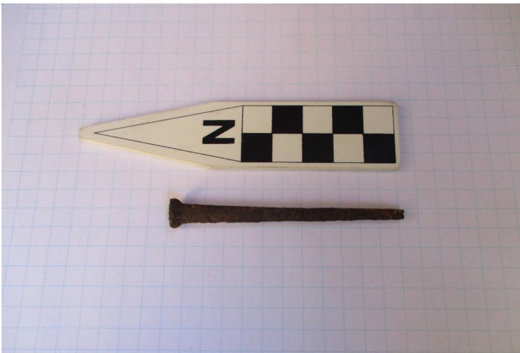
Photo 15. Detail view of Type 6 square cut nail found at northeast cabin, dates to ca.1830s; this type of nail was used throughout the presumed original part of the cabin (0271).
