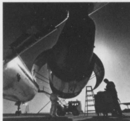
Synthetic lubricants are being used increasingly in jet engines. Emery esters of azelaic and pelargonic acids are important in the formulation of such synthetic lubricants.
