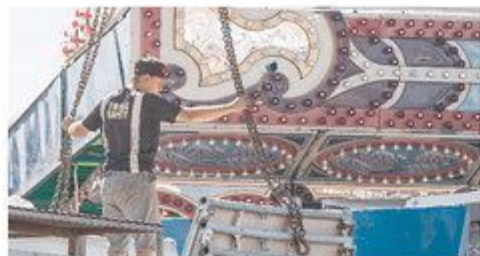
A fair worker secures hooks to a piece of ride equipment before it is hoisted off a truck.
