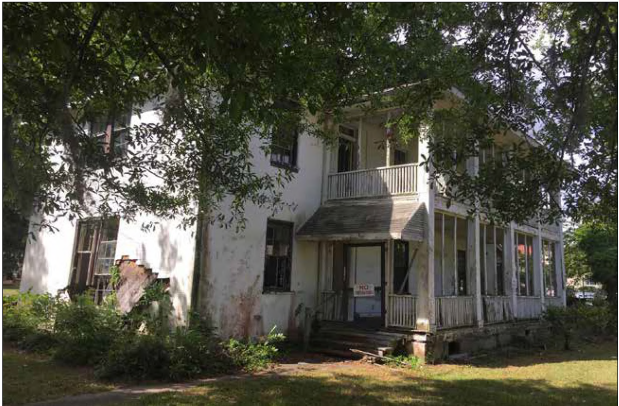
Figure 4.7 Medical Officer's Quarters (Building 763), northeast oblique, looking southwest. This is one of a pair of Medical Officer's dwellings that retains original architectural features, but is in a state of disrepair. Note the loss of structural framing at the window frame.
