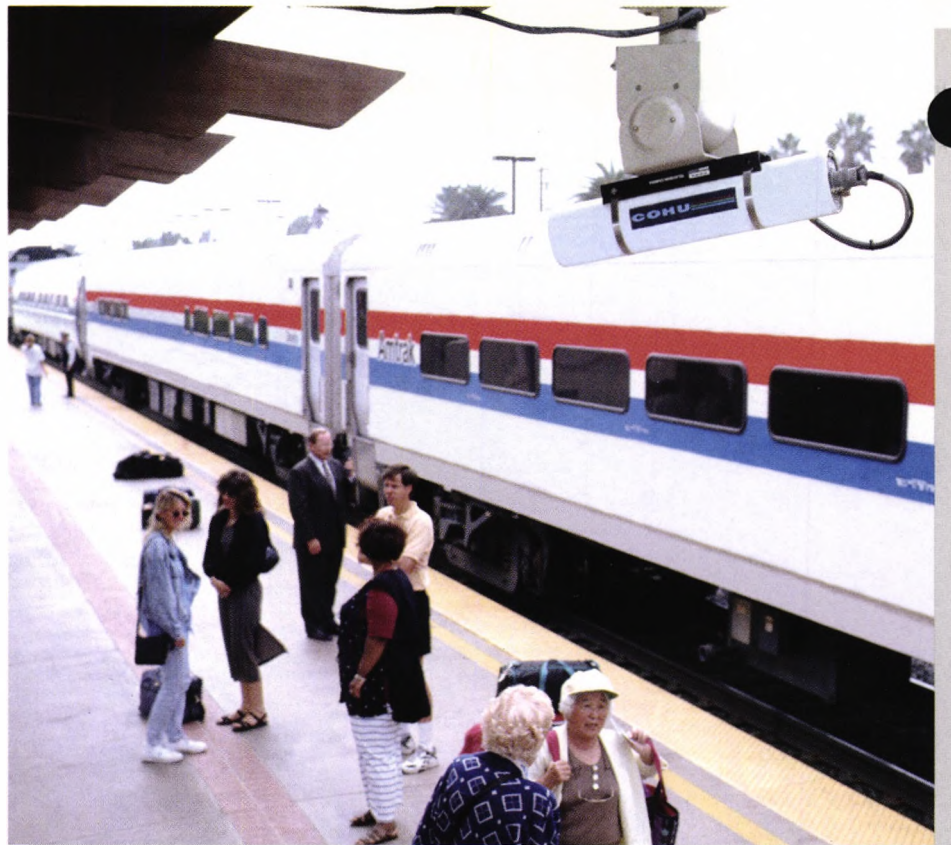
The Cohu cameras are enclosed in a pressurized housing to completely protect the cameras' internal electronic circuitry and lenses from adverse environmental conditions, especially the corrosive salt air from the nearby Pacific Ocean.
