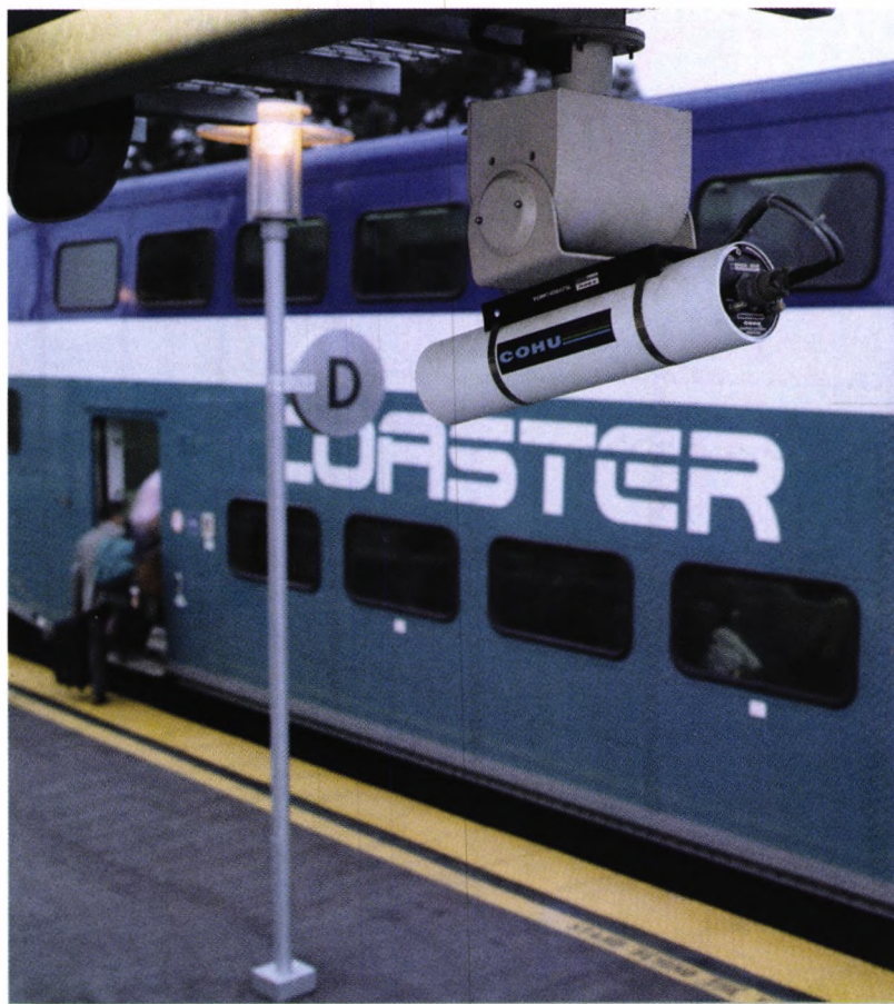
A color camera, mounted on a pan/tilt unit, gets a clear view of the platform and ticket vending machines. Parking lot cameras are monochrome.
