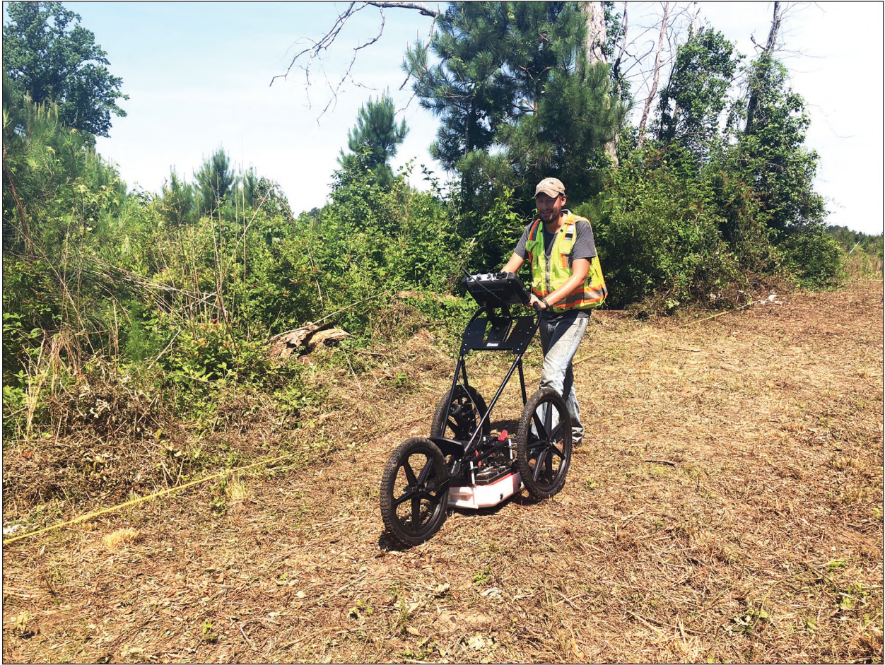
Figure 2. GPR Data Collection
