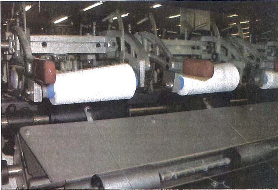
FINISHED PRODUCT. Automated equipment is used to wind yards of sewing thread onto spools at SarlaFlex. Each day the company produces thousands of spools of thread destined for companies throughout Central America, the United States and Canada.
