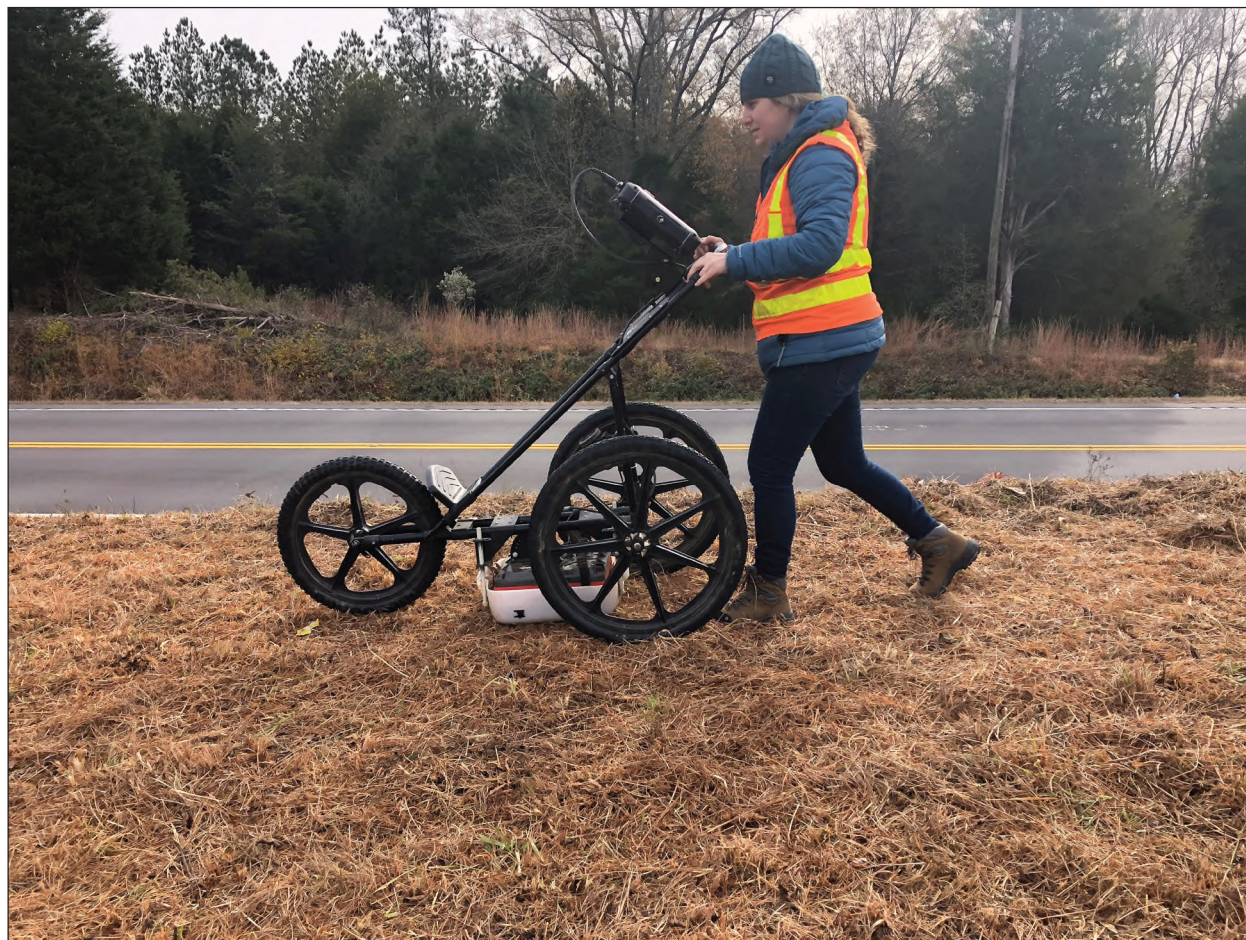
Figure 4. Photograph of GPR Data Collection in Progress
