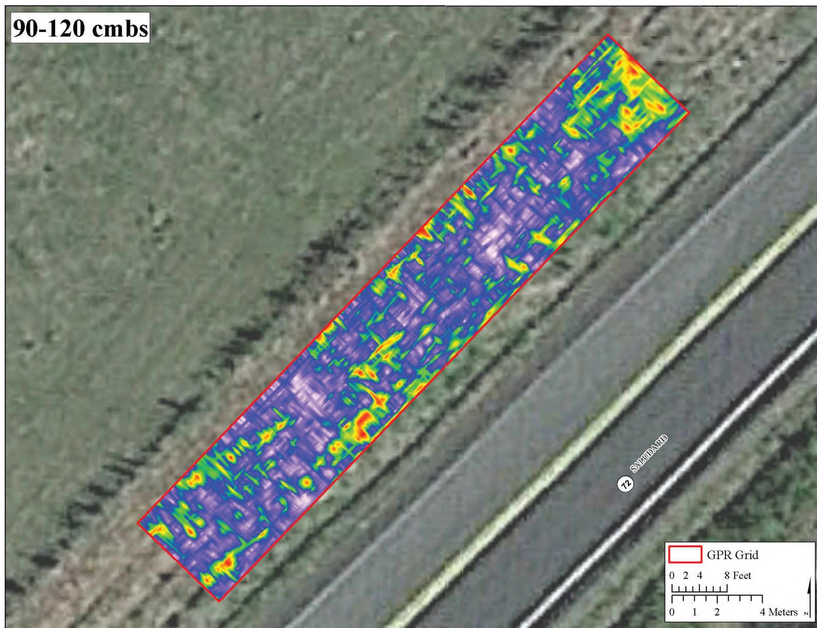
Figure 11. GPR Amplitude Slice Map, 90-120 cmbs
