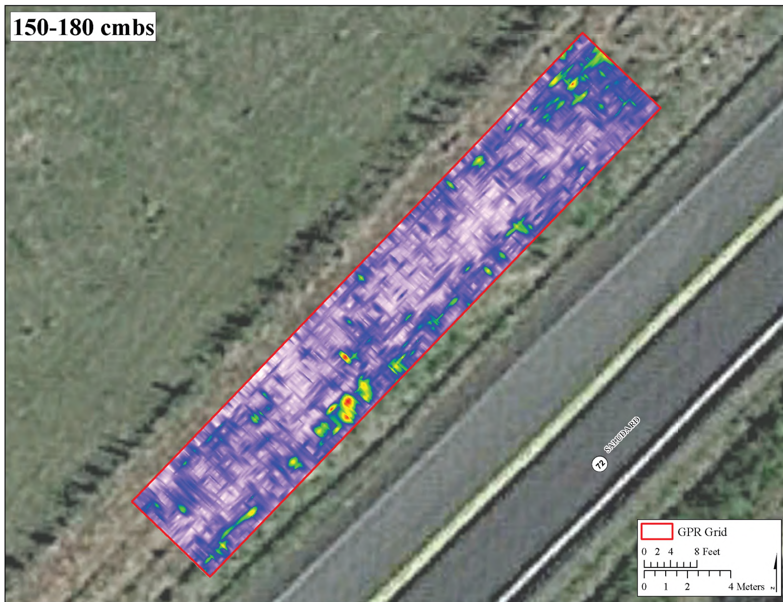
Figure 13. GPR Amplitude Slice Map, 150-180 cmbs
