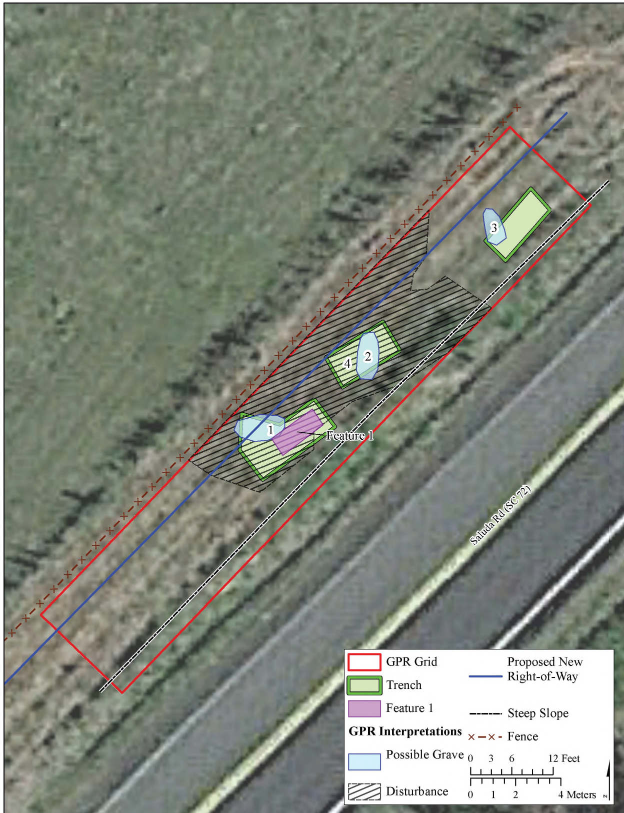
Figure 5. Trench Locations and Interpreted GPR Results
