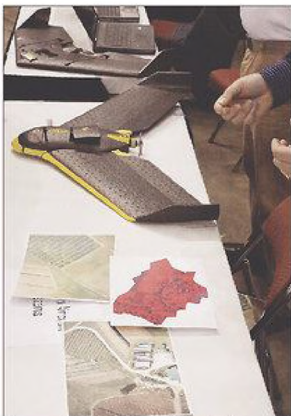
The unmanned aircraft displayed weighs less than 5 pounds and uses an auto-intelligent, pre-programmed pilot to maneuver. The aircraft can image 500 acres in about a half-hour.
