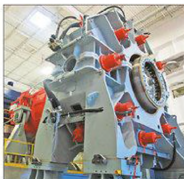
Gemson University's new Energy Systems Innovation Center in North Charleston features a 7.5 megawatt wind turbine testing rig. AP
